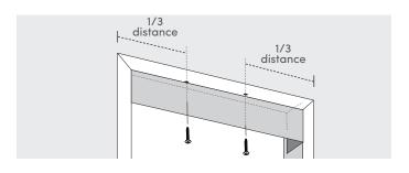
**B** – For OUTSIDE mount, **mark the location** of the shade mounting brackets with a pencil (see step 2), and measure 1/2" from the top of the bracket to note the location of the Valance bracket. Valance brackets should be installed 5"–8" from each end of the valance. Additional bracket(s) may be necessary and should be evenly spaced between the two ends brackets if required.
