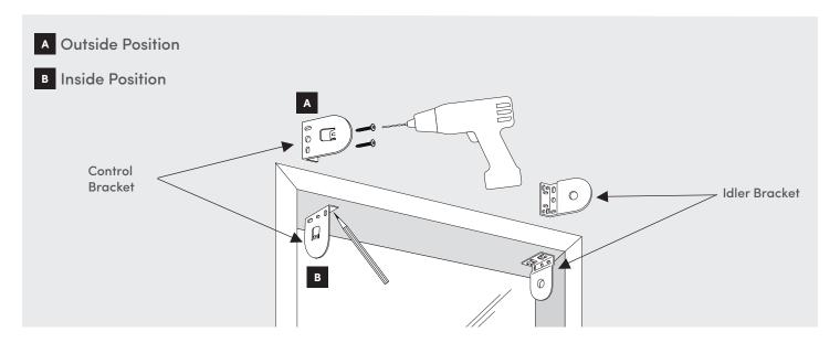
Inside / Outside Mount: Using a steel measuring tape, measure the distance from the outside edge of each bracket according to the ordered shade width. Mark the screw location on the mounting surface with a pencil ensuring these are leveled, snap end caps onto brackets (if ordered).
