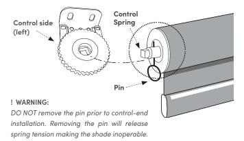
**B** - Insert the idler-end into the idler-end bracket. Ensure the control spring is compressed a minimum of 1/2" for proper operation.
