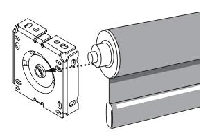
**B** - Hook the clutch side into the "+" shape of the clutch bracket.
