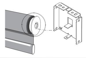
B - The idler end has a spring-loaded pin that allows it to compress in/out. Compress the pin and insert the idler-end into the idler-end bracket.
