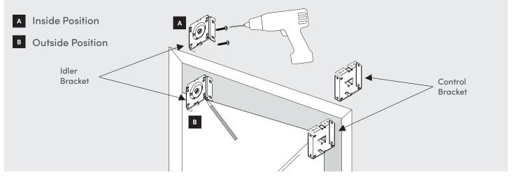
Inside / Outside Mount: Using a steel measuring tape, measure the distance from the outside edge of each bracket according to the ordered shade width. Mark the screw location on the mounting surface with a pencil ensuring these are leveled.
